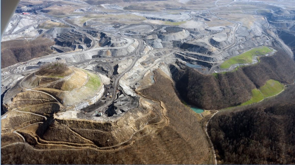
Figure 10. Mountaintop removal coal mining: the Twilight Mine complex 23 in West Virginia. (Photo courtesy of Vivian Stockman / www.ohvec.org ; flyover courtesy of Southwings.org.)
